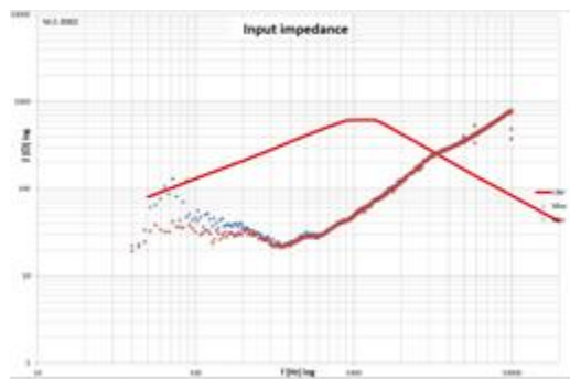
Figure 3. Dependence of input impedance on frequency of injected signal.
