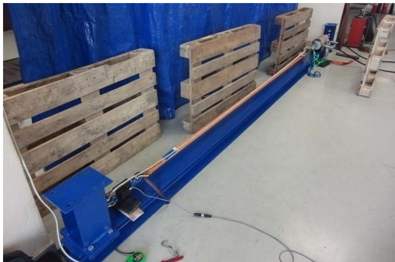
Fig. 1: Testing stand to test tension forces in lashing equipment
