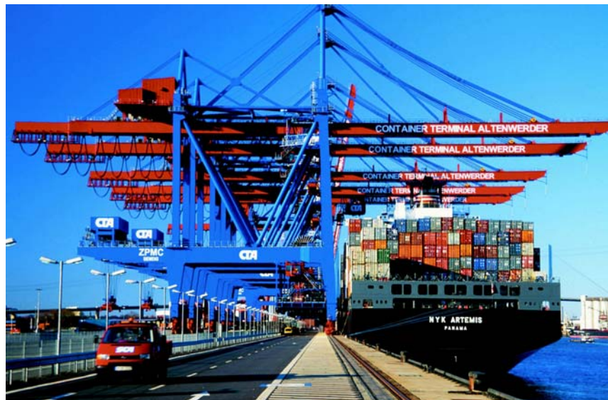
Fig. 1 - Semi-automated Gantry Cranes [1]
