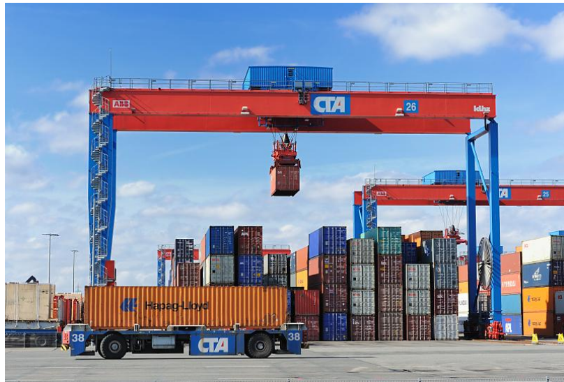
Fig. 2 - Automatic Stacking Cranes and Automated Guided Vehicle [1]
