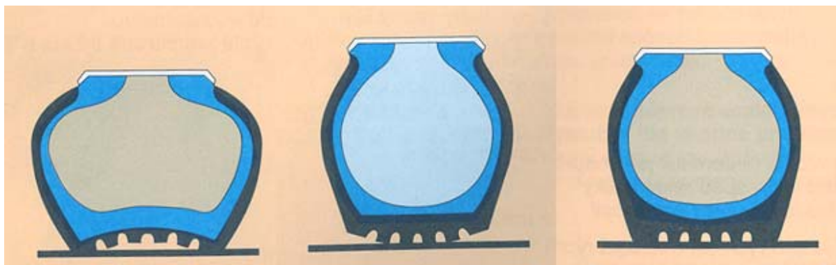
Fig. 3: The influence of underinflation, overinflation and the right inflation on the bald tyre (PETR CHVÁTAL: Autoškola CDE, Springer Media CZ s.r.o., ISBN 80-902549-7-7)
