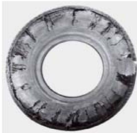
Fig. 2: Damaged tyre caused by their underinflation (firm literature Barum Continental, s.r.o. Otrokovice)
