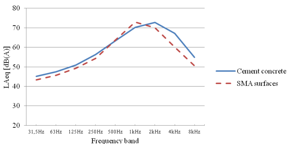
Fig.8. Spectral distribution of surface noise in case of a single car drive – at night, the measurement time 10 seconds
